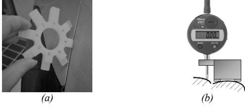
Fig. 2. Operators' devices for measuring gap and flush: manual feeler gauge (a) and dial gauge (b)
